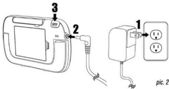
Press and hold the power button for 1 second to turn on the monitor unit. Power LED indicator emits blue light when monitor unit is turned on.
